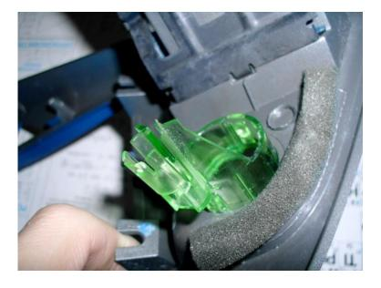
It should be at the top with a screwdriver press the plastic protruding, to remove towards the opening lighter.
