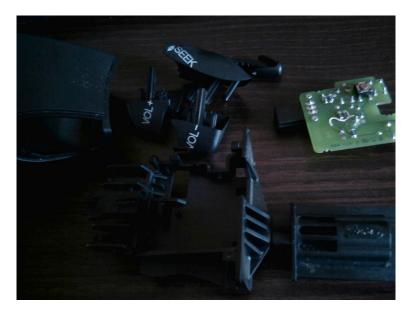
Then I started the modification of the electronic board. Remove old resistors, cut one cable, then I soldered new resistors in same place as old ones, and later a new ones combine with a short cable.
