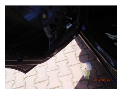
**9. We begin to suppress the inside** - first do the inner part between metal sheets. The first mat without cutting attach to the upper part, just below the window. Then Cutting squares, triangles, to do the largest part. Remember that everything stick tightly, without bubbles and without outliers pieces. So that in the future, not dropped out, or to not interfere during opening windows.
