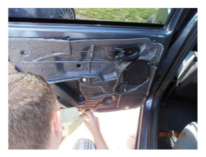
**5. Take off the handle** - already have a hole to put your hand inside and look for the plug is press fit of the handle. Gently grab from the inside. Push it out, so that the handle is intact.
