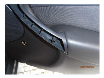
**3. Take off the cover handle** (if doors have electric windows unplug the connector from the cable), then cover the door gently lifting it up
